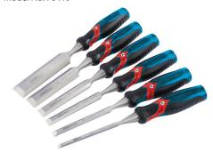
Expert Quality, full - length bevel edged blades manufactured from chrome vanadium steel hardened, tempered and finely ground. The solid impact - resistant soft grip handle allows the 'Pound Thru' striking end cap to be struck without causing damage. Supplied in an Content: 6 x chisels: 6, 12, 19, 25, 32, 38mm
