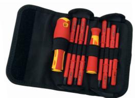
Expert Quality, tested to 10kV, suitable for working on live circuits of 1kV AC and 1.5kV DC. SCVM steel blades hardened, tempered and chemically blackened. nterchangeable insulated blades deep set into handles - precision or high
